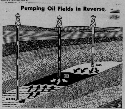
PITTSBURGH, PA.—By pumping water and natural gas into the depths of the cil fields, modern science is bring 10 to 50 per cent more oil to the sur ace. This typical cross section shows one way it's done. Here g. pumped in above the oil pool, and water underneath it. These artificial pressures, from above and below, force the oil to flow thru the sand or rock in which it is imbedded and up the well shaft. Sketch is based on an explanation by Gulf Oil.
