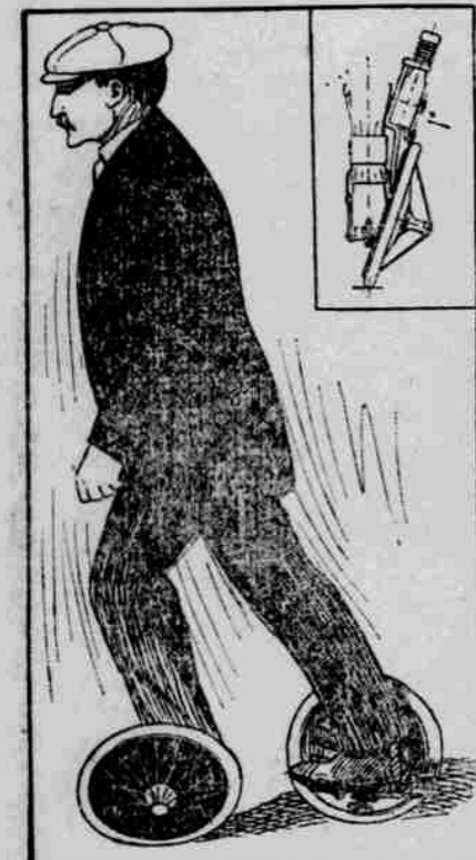
A Skater and One of the Skates with Motor Attached.
