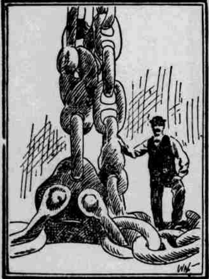
Moorings-Chains for the New Cunarders. The Largest Chains in the World.
