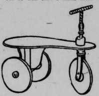
you may also like to make one to give away. I used a piece of beaver board and first cut out the seat and the wheels and then put it together with wire and spools. I made a handle to steer the front wheel. It runs well and will last quite a little while if not handled too roughly. Your friend,
