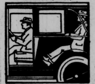
Front seat adjusts to three positions to accommodate short driver or tall driver.
