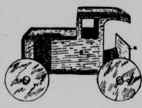
your curves at front of box, leaving part for the dashboard. The wheels are made of quarter-inchwood with flat rubber bands stretched round the rims for tires.
