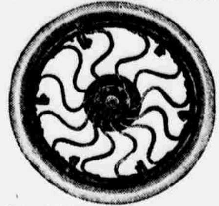
Automobile Wheel With Spring Spokes and Sectional Fellyes That Move In and Out to Adjust the Tire to Irregularities in the Road.
