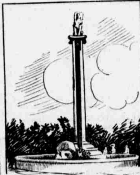
Barometer Which Contains Column of Olive Oil 37 Feet High.
