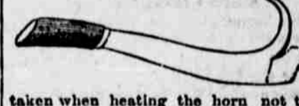
taken when heating the horn not to heat the blade so as to draw the temper.
