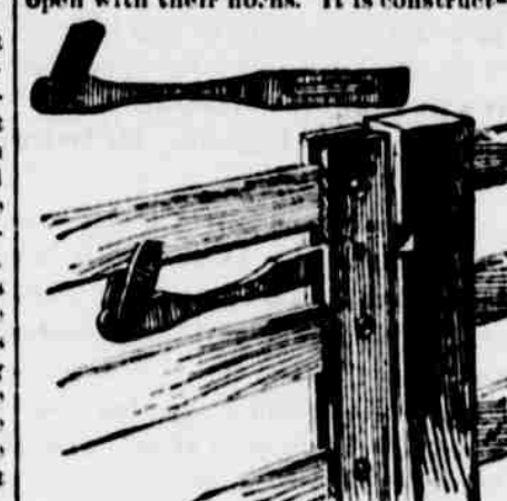
A New Jersey friend sends a drawing of a gate fastener. The wind can not jar it open, neither can cattle push it open with their horns. It is constructed the same as the ordinary slide latch, except that it has at one end two levers fastened to it and the gate. At the other end is a slot, through which a bolt works, fastened in the gate. The illustrations plainly show how any one can construct it. —Farm and Fireside.
