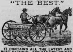
IT CONTAINS ALL THE LATEST AND BEST PATENTS, AND HAS NEW POINTS OF EXCELLENCE DFFERED BY NO OTHER DRILL. IT CHANGES FROM SINGLE TO DOUBLE RANK INSTANTLY AND WHILE IN MOTION. IT HAS A FORCE FEED GRASS SEED SOWER, A NEW FEATURE. WE ARE PREPARED TO SHIP DIRECT TO PARTIES IN LOCALITIES WHERE WE HAVE NO AGENTS. Parties ordering, will please say in what paper
