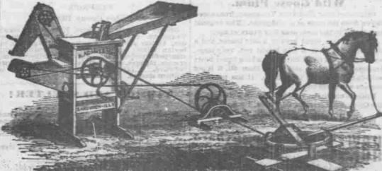
Two Hole Self Feed Sheller, with single sacker, two-horse power, geared ...
