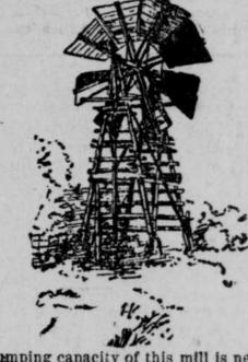
pumping capacity of this mill is nearly one thousand gallons per hour in a fifteen mile wind. The description and illustration of this windmill were taken from Bulletin No. 59 of the University of Nebraska, which is exclusively devoted to home-made windmills.
