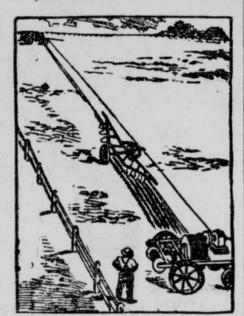
ELECTRICALLY OPERATED PLOW. field. The mechanism is so adjusted that when once set in motion the apparatus practically operates itself. moving the carriages forward at the beginning of each trip to bring the plowshares in position for the next row of furrows.
