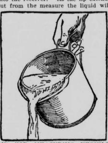
LIP FOR MEASURING VESSELS. not run down the outside either at the beginning or end of the pouring, and, the lip being perfectly plain, it is an easy matter to wipe it dry.
