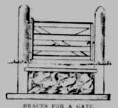
of heavy studding may be run from the bottom of each post next to the sill up to the top piece of studding; the stone wall, as suggested, makes the stronger foundation. Built in the manner indi-
