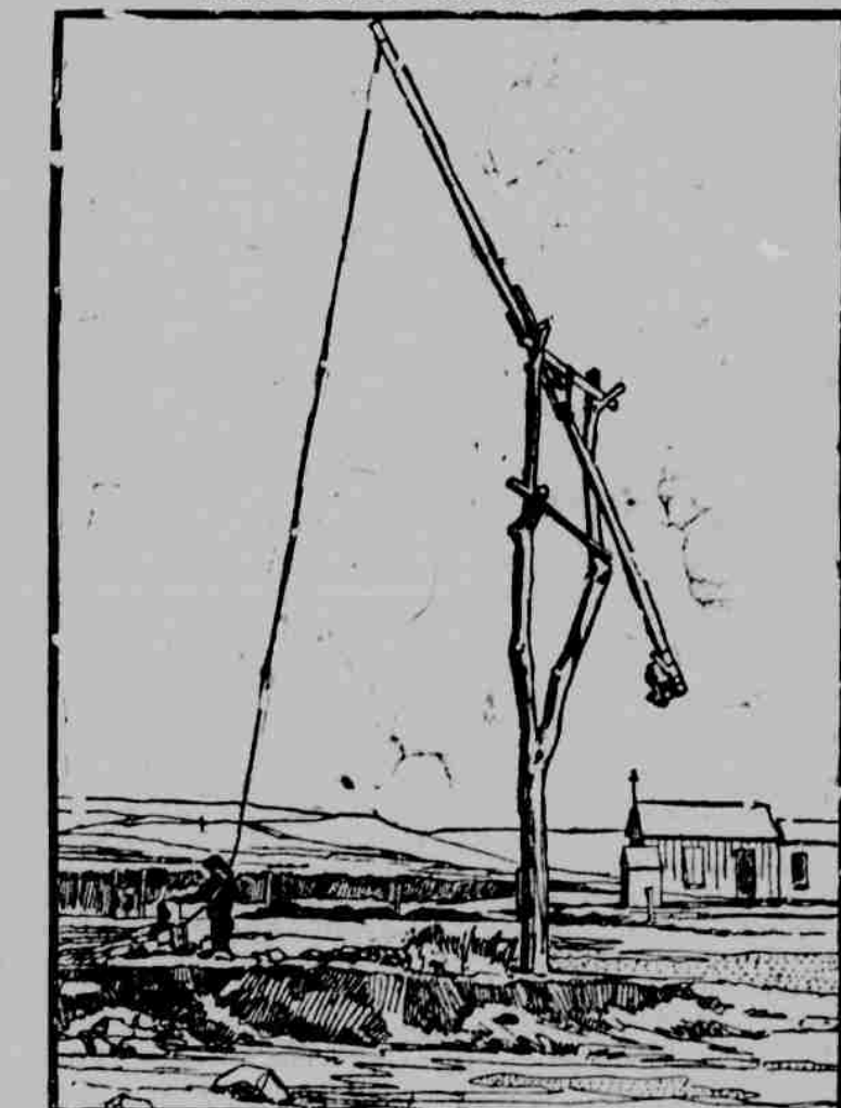
Near the little town of Tia Juana, just across the boundary line in old Mexico and near the Pacific coast, there is a very curious well. The inhabitants of this country seldom go far away from their homes and they have very primitive ideas and customs. This well is about 50 feet deep, and the owner has built an ingenious device for hauling water from it. If this Mexican had been an educated man he might have been an inventor. A tree flourished near the well which had two branches growing out of the
