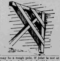
hand, though the pole should be stout. Such stagings are useful where one does not wish to mar the shingling or clapboarding by nailing on boards to build the usual stage. Besides, these frames can be laid aside ready to be put up again at a moment's notice, proving in this way a saving of labor.-American Agriculturist.
