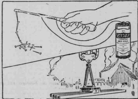
EVERY boy is familiar with the is dated, and therefore fresh and which picks up nails, needles, and wound around the metal part of the other metal objects and makes screwdriver, as shown in the illusthem act as if they were bewitched. tration, and the ends are connected But a magnet can be made in a to the battery. few minutes which will furnish | The operator then takes hold of
