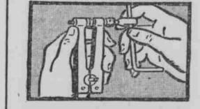
Assembled instrument. Split bearings and shaft, lubricated with competitive oil, are clamped between "jaws" of instrument. With set-screw, extreme pressure is applied.
