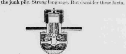
No matter how carefully piston rings are fitted, or how finely the carburetor is adjusted, gasoline vapors leak past the piston rings. Besides this, oil is contaminated by hard particles of road dust drawn in through the carburetor and the breather tubes. After 500 miles of operation, crank-case oil is becoming a grinding solution. With such oil rapid wear
