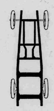
The Special-Six chassis frame is 7" deep. It tapers from a width of 29" in the front to 41" in the rear, so that the sides of the bodyfit perfectly without overhang. Five crossmembers prevent the dis-tortion that eventually causes bodies to squeak
