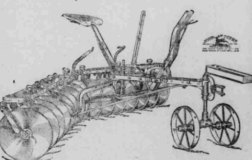
Instant Leveling for All Conditions-Enabling operator to keep all discs cutting an even depth.
