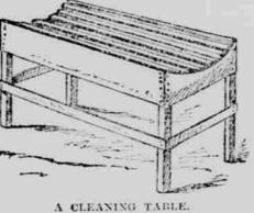
The second cut shows a cleaning table. It is made with a slightly curved top to prevent the carcass from rolling off. Its construction is easily soon. The slats on it are 1x2 inches, set on edge and firmly spiked down to the two curved end pieces. It is a very convenient table for cleaning hogs before hanging up, and, indeed, for cleaning and washing almost anything.
