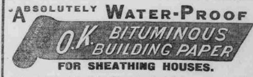
We call attention to the novelty of its construction, it being composed of two sheets of paper with an interposed layer of water-proof bitumen or asphalt, the whole united under pressure, making a sanitary mildew-proof sheathing for the sides and floors of houses, that will last as long as the building upon which it is applied.
