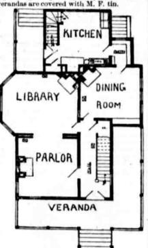
FIRST STORY PLAN. The floor of atticis of dry 3/4x4 tongued and grooved spruce; the floors of veranda and porch of 1½ white pine; all other floors of ½x3 yellow pine, blind nailed. The kitchen, bathroom and pantry, treads and risers of front and back stairs, of yellow pine. All other inside woodwork of white wood.
