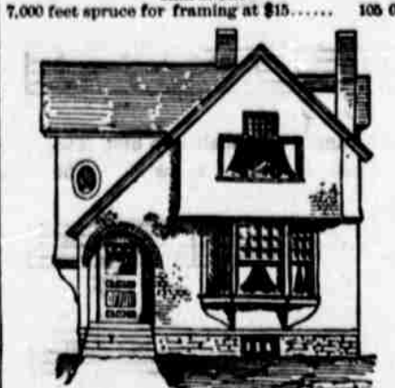
FRONT ELEVATION. 4,000 feet hemlock boards at $12, 46 square cedar shingles at $4, 1,600 feet spruce flooring at $20, etc.
