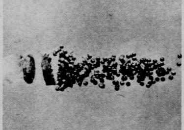
The high-speed photograph above shows the shot charge from our plastic shell when it's three feet from the muzzle. Note the short, uniform stringing and good distribution. You get this because our friction-free, plastic-against-plastic design seals powder gas perfectly. There's no escaping gas to scatter or disrupt the charge. Result: better patterns, longer range... thanks to all-plastic construction.
