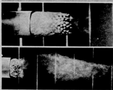
The photographs above show two shot charges as they leave the barrel. The top one is from our plastic shell; the other, from a paper shell. Notice how the powder gas in our plastic shell stays behind the shot, pushing it with maximum power and velocity. The powder gas from the paper shell has leaked past the wad into the shot, weakening the shot charge—proof that only our plastic wad in a plastic body gives you all the power you paid for.
