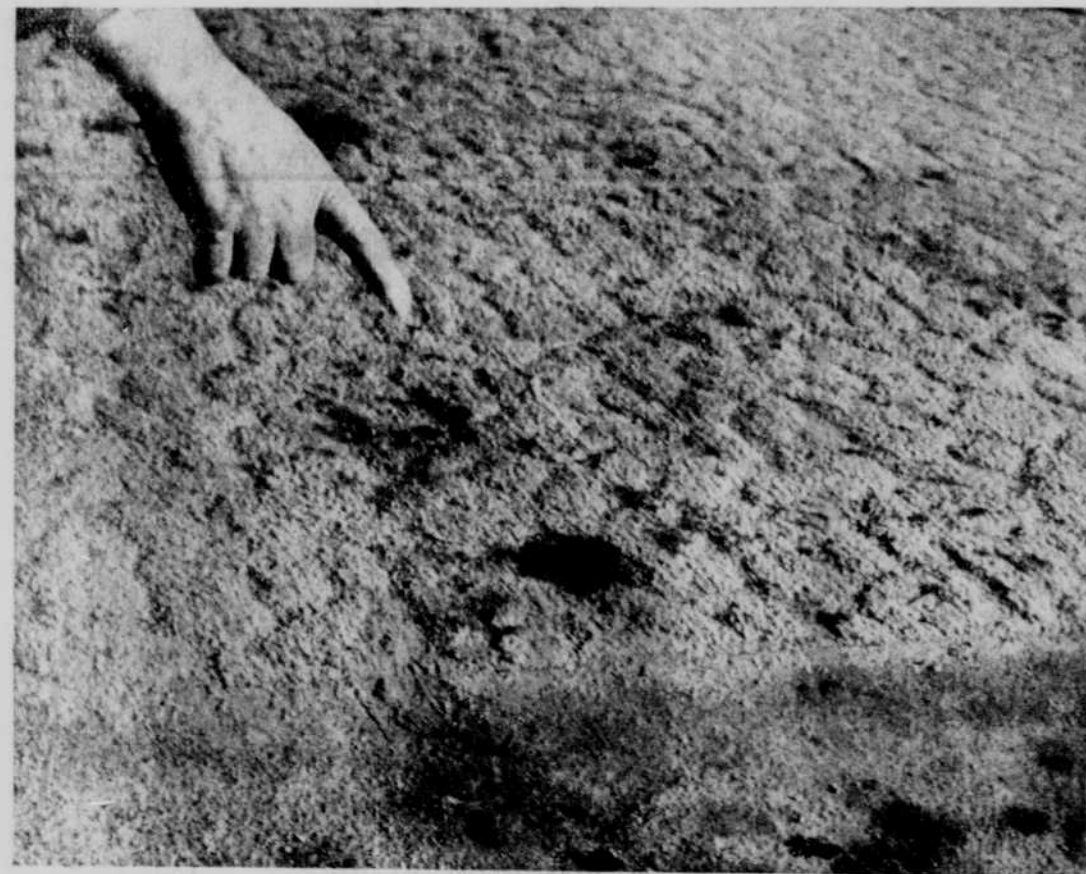
Here the carpet is after one week of heavy traffic, including trucks, cars, mud, sand and soil. The heavy black spots are oil that has dripped from cars while being serviced.
