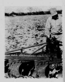
When a mounted plow won't opera will have to adjust the top link as be discussed in your implement mar using a mounted plow is the spacin don't, the front bottom will be cuttin. These mounted plows will have a may need to be changed from time.
