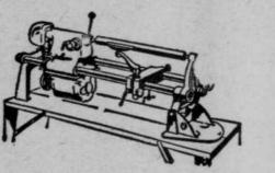
multi-purpose SHOPSMITH in action -as a circular saw, a disc sander, a wood lathe, a vertical or horizontal drill press!
