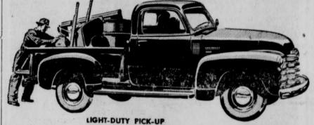
Madel 3104-116-inch wheelbase, Maximum G.V.W. 4,600 lb. Other models available: 3604-1251/4-inch wheelbase, Maximum G.V.W. 5,800 lb; 3804—137-inch wheelbase, Maximum G.V.W. 6,700 lb.
