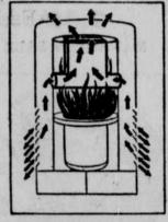
Only the Heatrola has the famous, patented Intensi-Fire Air Duct. Built right in the path of the flame, it blocks much of the heat ... sends it out into the rooms instead of up the flue.
