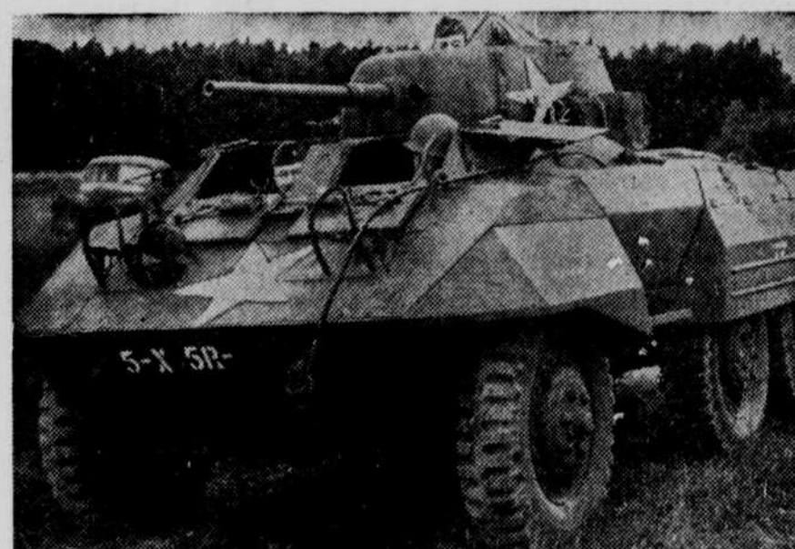
This is the armored car, M8, latest combat vehicle addition to the army's mechanized equipment. Designed by ordnance department to combine speed of the auto and punch and protection of the tank, debut discloses M8 as six-wheeled, weighing eight tons. It mounts 37-mm. cannon and .30-caliber machine gun and is manned by a crew of four.
