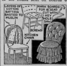
plywood. Cut out the wooden seat and screw it to the chair. Save the cardboard pattern.
