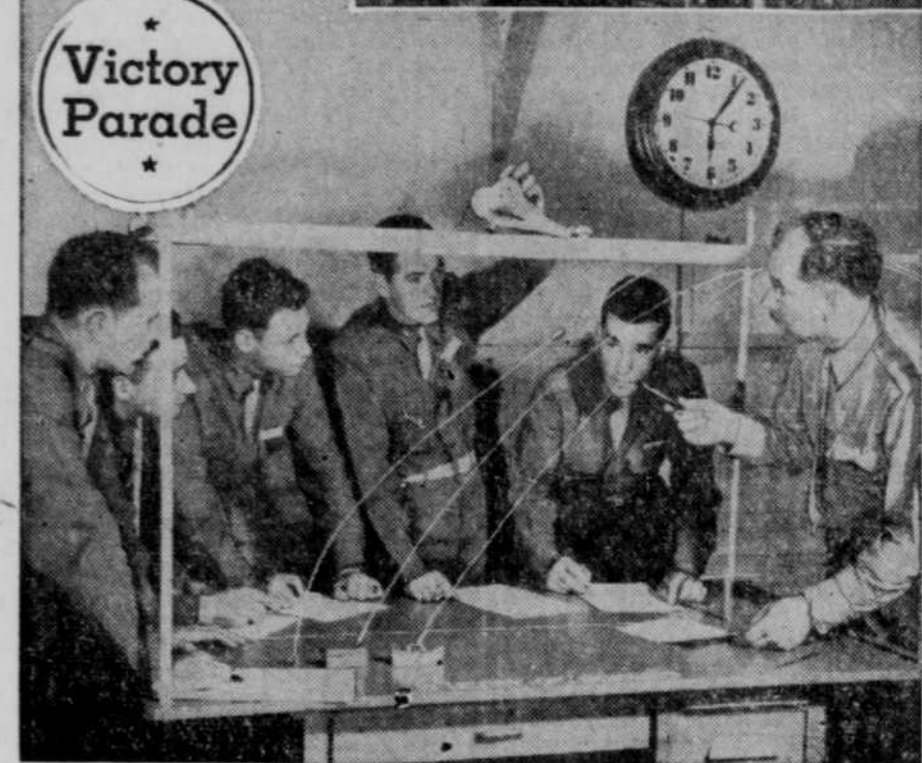
Synthetic trainer. Miniature plane slides along track at top, releasing toy bombs along wire tangents.
