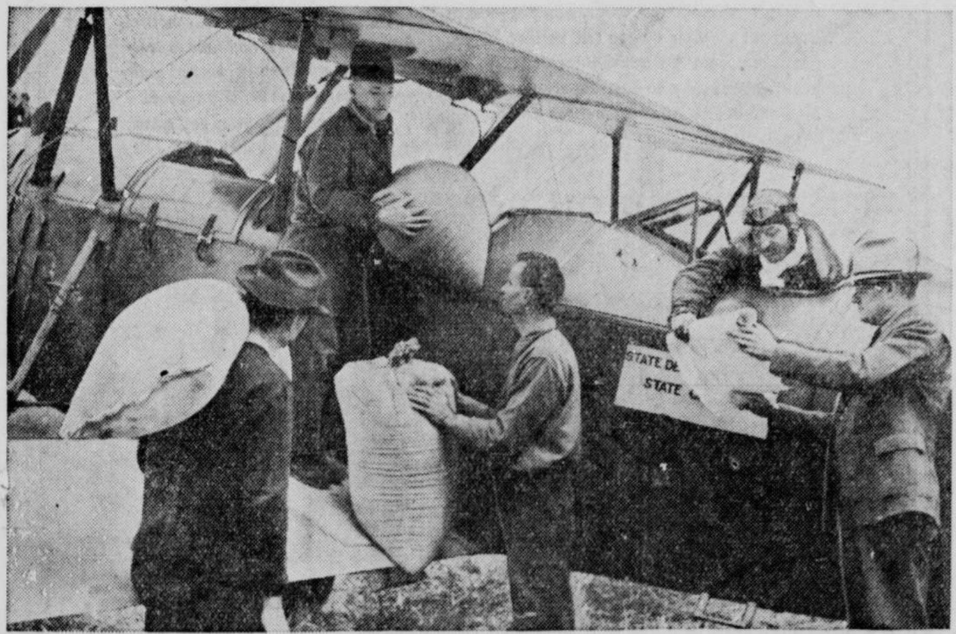
One of the former mail planes used by the government which is now being used to scatter seed over burned-over forest land. The compartments once used for mail have been rebuilt as seed bins with trap doors in the bottoms which can be released by the pilot. The planes carry about 800 pounds of seed.
