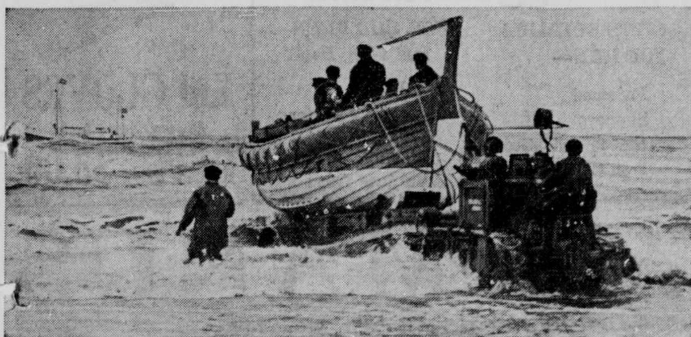
A new method of launching coast guard boats into surf is demonstrated on the coast of Holland. The equipment includes a tractor with caterpillar drive and a special truck for the boat.
