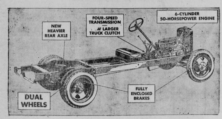
Light Delivery Chassis . \$365 Light Delivery Chassis with Cab ..... \$470 (Pick-up box extra) Roadster Delivery ... \$440 (Pick-up box extra) Sedan Delivery . . . . . 5595 with Cab . . . . . . . . . . \$625
