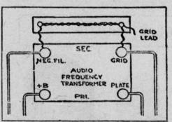
When static is real bad the strength of the leak can be increased to where it will take the harshness out of the static, but it will reduce the signals somewhat.
