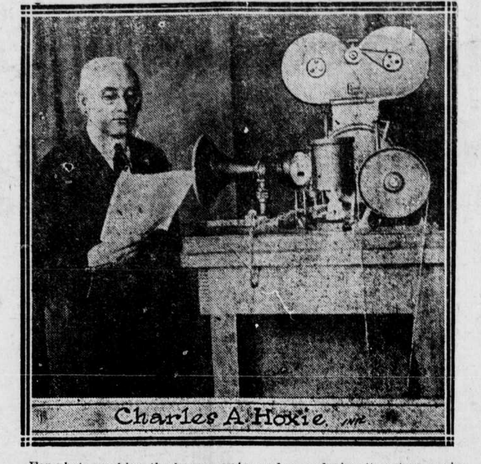
Charles A. Hoxie. For photographing the human voice and reproducing it, not as a picture, but as the sound of the voice itself, a new device, known as the Fallo-Photophone, has been perfected by Charles A. Hoxie, of the General Electric Co., Schenectady, N. Y. It is believed the machine will make the talking-motion picture a reality.
