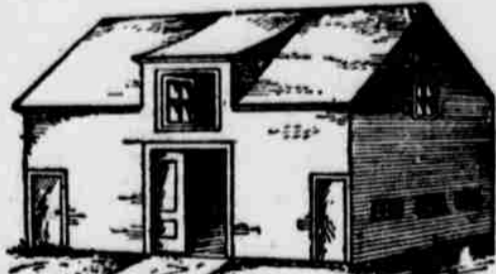
THE IMPROVED BARN. of window that is shown is much better than the pitched roof dormer window that is sometimes put upon roofs. The style shown admits of having a large square window in front—especially useful if a hay fork is to be used.
