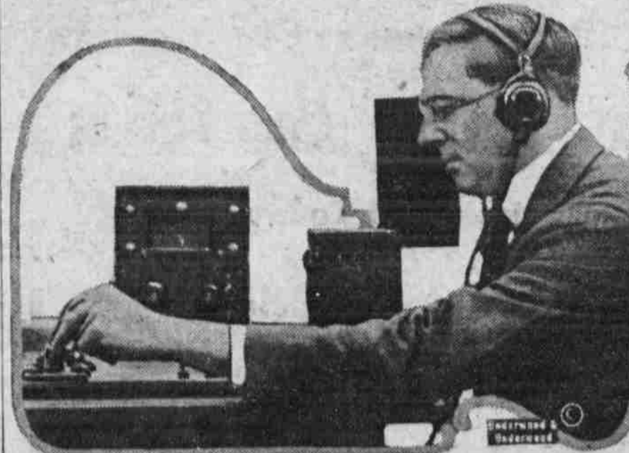
Earl C. Hanson, American inventor who served in the navy department of engineering during the war, with the receiving apparatus of his new invention on the United States torpedo boat destroyer Semmes, while his apparatus was guiding the vessel through Ambrose channel. An apparatus on the ship receives impulses from a submarine cable laid for the purpose. Hanson invented an amplifier which renders the electric signal currents as understandable as a telegraph message. Receivers on each side of the ship give out sounds through ear pieces so the navigator can tell by the loudness of the sound in each ear when he is over the cable.
