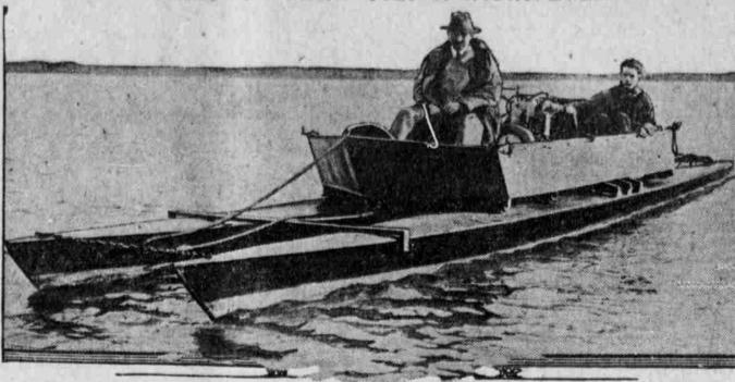
Vivian Nickalls, the English coach of the oarsmen at the University of Pennsylvania, is using a fast hydroplane of the catamaran type to keep alongside or ahead of the racing crews at practise. It makes little wash and is better adapted to the work than an ordinary launch.
