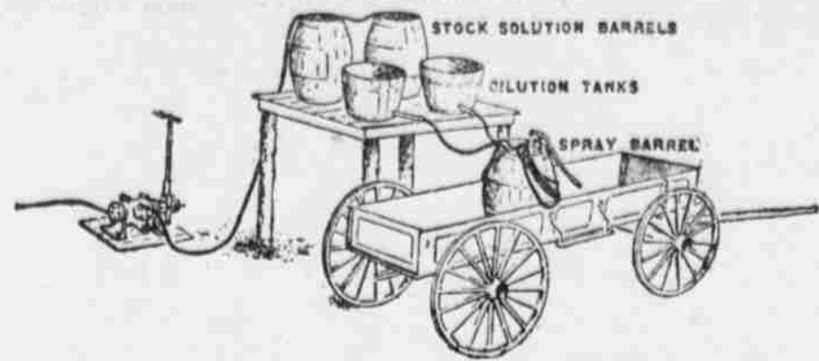
Cheap and convenient mixing platform for making Bordeaux mixture.
