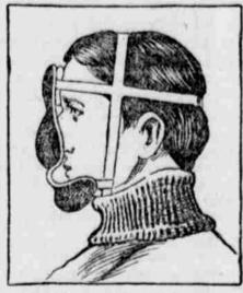
to the right tension, and the cup-like chin portion of the guard prevents any side motion or accidental displacement. As the guard does not come in contact with the mouth or nose it will not interfere with the breathing in the
