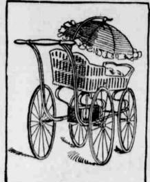
mechanism consists of a spring motor properly encased to hide as well as protect its working parts. A large drum revolved by the spring is connected to the bottom of the coach by a shaft, which, as the drum turns, imparts a rocking motion to the body of the carriage. Means are provided for starting or stopping the machine at
