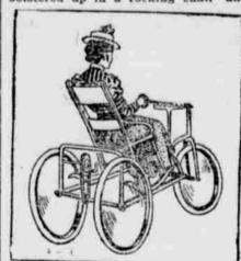
rocks himself back and forth. motion of the rockers, which rest on springs, is translated into a rotary motion which operates the sprocket wheel and chain and this in turn operates the driving wheels in the rear. The latest achievement of inventive genius will at least aid in developing the abdominal muscles, and, as this is a weak spot in the present generation, perhaps the rising generation in the west will be exhibiting wonderful development in this region.
