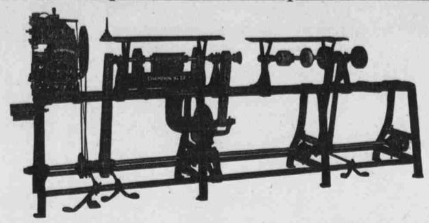
Above is a cut of the new CHAMPION QUICK REPAIR MACHINE for sewing, half-soling and finishing shoes, which arrived this week and has been installed in
