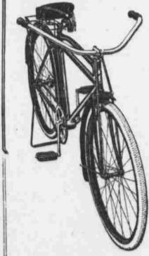
It has a 20-inch Frame with Coaster Brake. Motor Bike Handle Bars, Eagle Diamond Saddle, Motor Bike Pedals, Motor Bike Grip, Luggage Carrier Holder, Folding Stand, Front and Rear Wheel Guards, Truss Frame and Front Fork.
